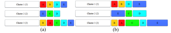
Figure 15. Simplified visualization of raw process traces. Each row is a cluster's prototype. The information in the white block before the prototypes shows the cluster ID that each prototype represents and the number of process traces in that cluster. (a) Cluster prototypes are consensus sequences calculated from context-aware alignment (Figure 9(a)); (b) Cluster prototypes are consensus sequences calculated from duration-aware alignment (Figure 9(b)). The data comes from Figure 4.
